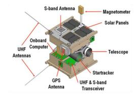
Figure-3: 3U CUBESAT with telescope Figure-4: Internal Components of a CUBESAT
